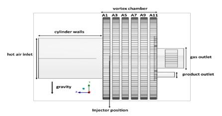
Figure 1. Geometry of vortex chamber spray dryer
