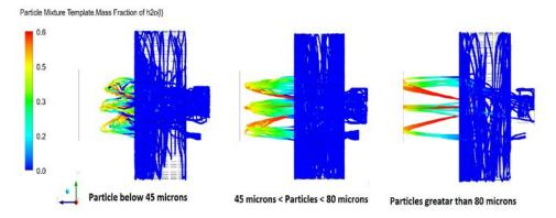
Table 2, shows an overall drying performance as discussed by Huang et al [14]. Some of the particles are trapped in circulating zones and do not escape. These are removed from calculations after 10 seconds.
