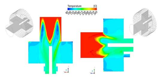
Figure 6. Temperature patterns on two axial planes, with water spray
