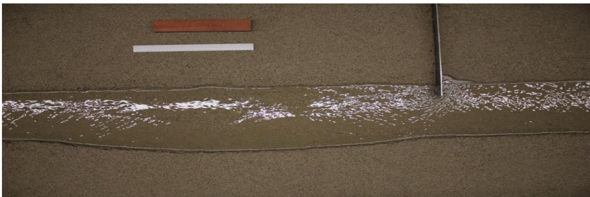
Figure 1. Opposite bank erosion with spatial lag (flow from right to left). Bonilla-Porras (2017)
