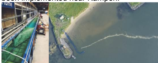
Figure 2 Testing the Great Bubble Barrier in the lab and in the IJssel (picture: TGBB)
