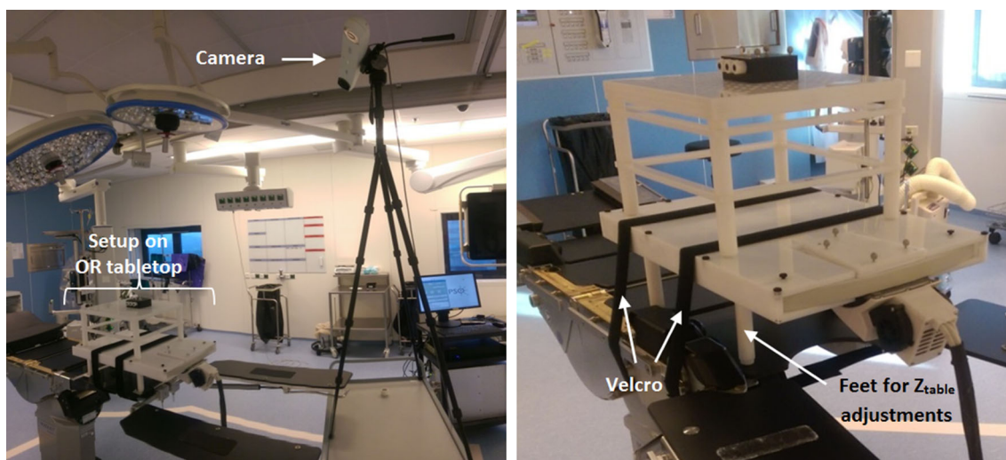
Fig. 2 Setup for OR measurements. On the left a picture showing the complete setup environment and camera position. On the right a zoomed in picture of the measurement setup fastened on the OR tabletop with Velcro and showing the feet to adjust Z_{\text{Table}}
