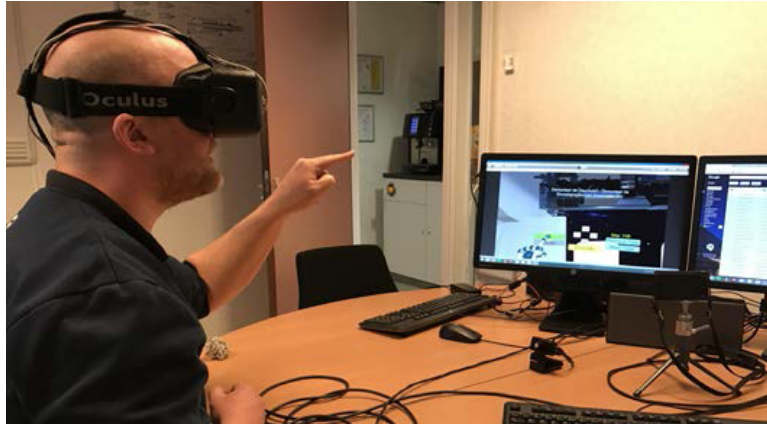
Figure 5 Set-up of the workspace with the leap motion sensor combined with the HMD oculus DK2 during the testing phase in Maastricht service location (see online version for colours)
