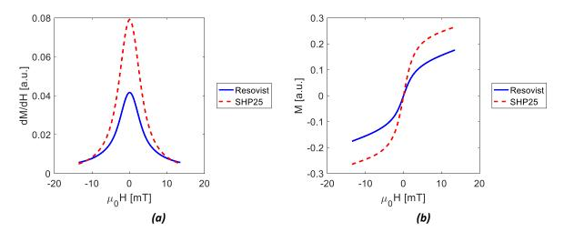
Figure – SPaQ results, measured on Resovist (Bayer Schering Pharma GmbH) and SHP-25 (Ocean Nanotech) samples containing 750 µg iron in a total volume of 150 µl, at a frequency of 2.5 kHz. (b) is a numerical integration of (a).
