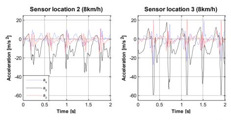
Figure 8. Example of clipping. Example of raw accelerometer data, while jogging 8 km/h. (Left), sensor location 2—no clipping. (Right), sensor location 3—clipping on one axis at 6 g.
