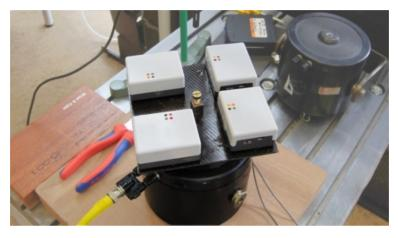
Figure 6. Setup of the sensors on the mechanical oscillator. Four ProMove2 sensors were securely fastened to a mechanical oscillator (Vibration Exciter, type 4809, Brüel & Kjær).
