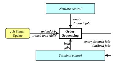
estimated time at which the (consolidated) order will be ready for processing. Order sequencing triggers empty AGV assignment and dock assignment to search for resource capacities to handle the jobs.
