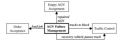
Figure 5. AGV Failure Management related to the other local control objects
