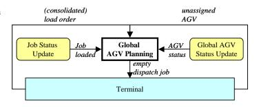
time that an empty vehicle has to leave the terminal in order to arrive on time at its destination. If too early arrival at the destination is not allowed (e.g. because the storage capacity at the destination is small), an order may be given an *earliest dispatch time*. Input to the decision process are (1) consolidated order lists from the terminals and (2) AGV status information (position, current order). The terminals confirm loading of orders to update the order list of global AGV planning.
