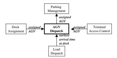
assignment or by terminal access control. The goal seeking heuristic proceeds from the earliest and latest time at which the AGV is allowed to arrive at the dock (see Dock Assignment). The agent calculates the earliest and latest dispatch time from its current location using an offset for the travel time. If the AGV cannot be dispatched immediately, parking management is triggered to find a solution.
