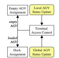
without hindering other traffic (parking management, dock assignment), and (2) the total number of AGVs driving on the terminal does not exceed some predefined threshold. It is triggered by AGV status updates. The agent bases its planning on an overview of the expected times at which AGVs will arrive at the terminal entrance and the expected times at which AGVs will leave the terminal.
