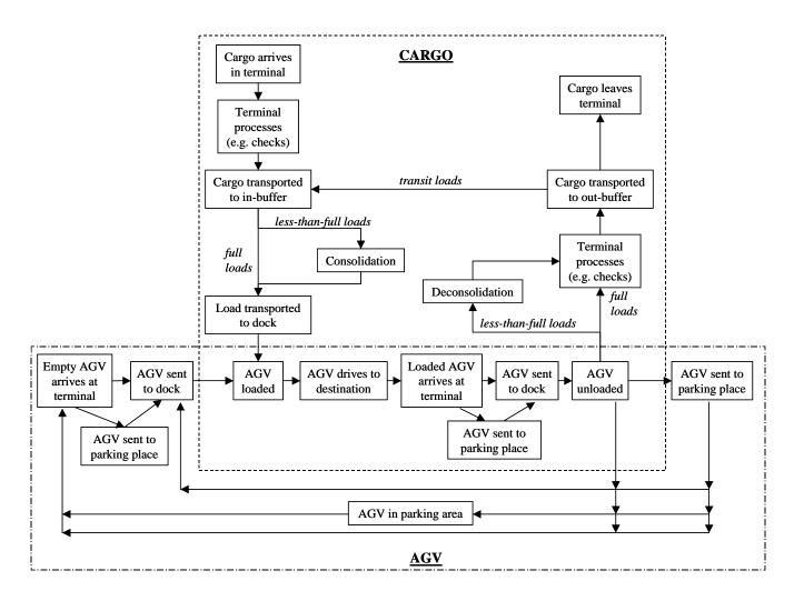
Figure 2. Physical primary process in an automated transportation network
