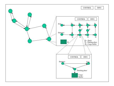
Figure 1. Example of an automated transportation network
