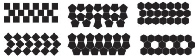
Fig. 18. Exploration of basic shapes for the garden fence module: square, rhombus, pentagon, and hexagon. In the prototype, the hexagon was used.
