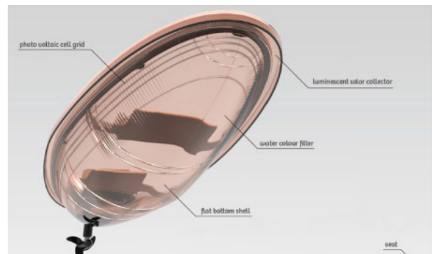
Fig. 9. (Color online) LSC transparent sculpted hull design with PV cell grid by Jullian Claus, Rosan Harmens, and Hieu Nguyen.
