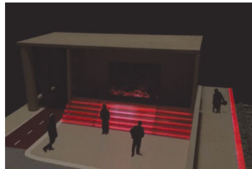
Fig. 14. (Color online) Application example of LSC illuminating safety strips concept by Ashley Hogt.
