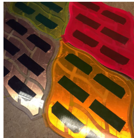
Fig. 1. (Color online) Various differently colored prototypes of Leaf Roof LSC PV modules. 13)
