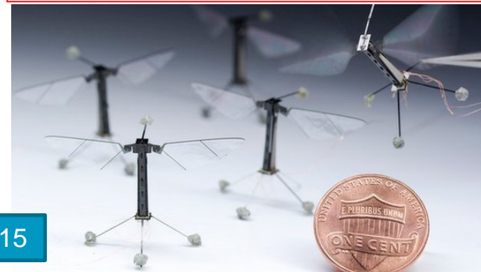
robo-fly, developed at Harvard, weight < 1g
