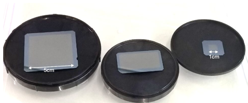
Figure 10: First larger scale (11 and 25cm 2 ) metal silicide samples
