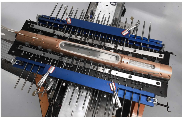
Figure 5. Photograph showing an overview of Feather-M2.1 during coil winding. Visible are the individual turns, the copper spacer and ring, the former and the winding and impregnation tooling.
