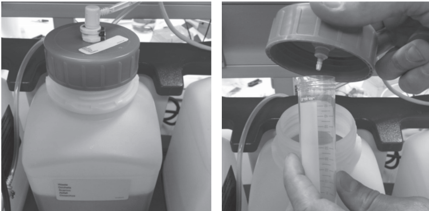
Figure 1. Manual waste collection from the CellSearch Autoprep by unscrewing the top from the waste container (left) and collecting the sample in a 50 mL Greiner tube.
