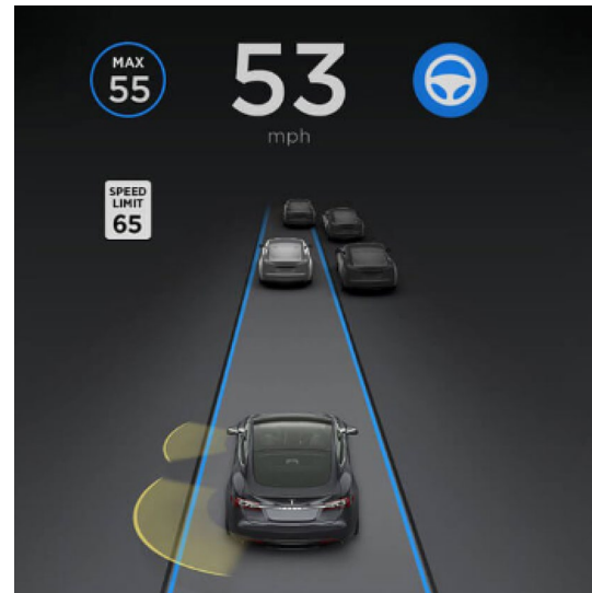
Fig. 2 T Model S with latest update of extended Autopilot function (version 8.1) showing a detailed image of what the vehicle sees around it (copyright Tesla.com)
