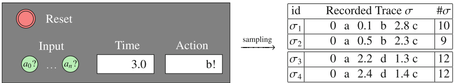
Fig. 3. Black box timed trace machine with input alphabet a_0?, \dots, a_n? , reset button, and time and action windows. Running the machine m times and observing traces of length k yields a sample. The ID together with the trace and the respective number of occurrences are noted down.
