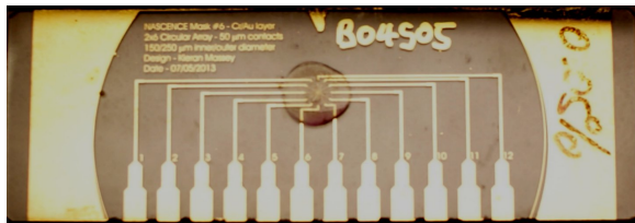
Fig. 8 Circular twelve electrode array with a mixture of SWCNT and PMMA in the centre [42]
