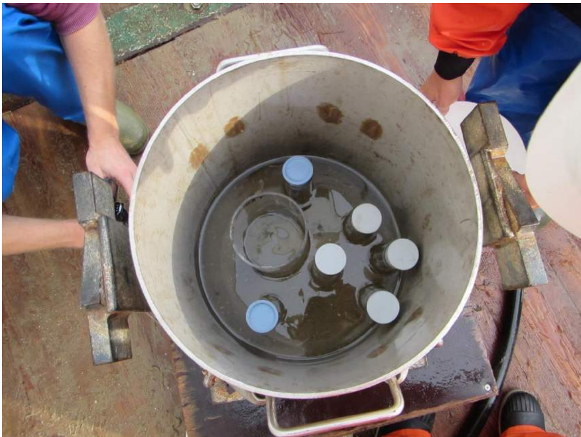
Figure 1. Sediment collected from the North Sea using a 30-cm-diameter boxcore, with subsamples taken for sediment analyses (photo: C. Cheng).
