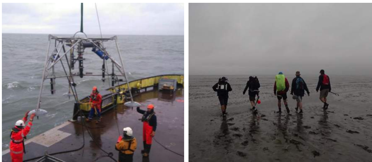
Figure 1. Installation of a main frame on the ebb-tidal delta (left). Installation of flow meters on a tidal divide (right).
