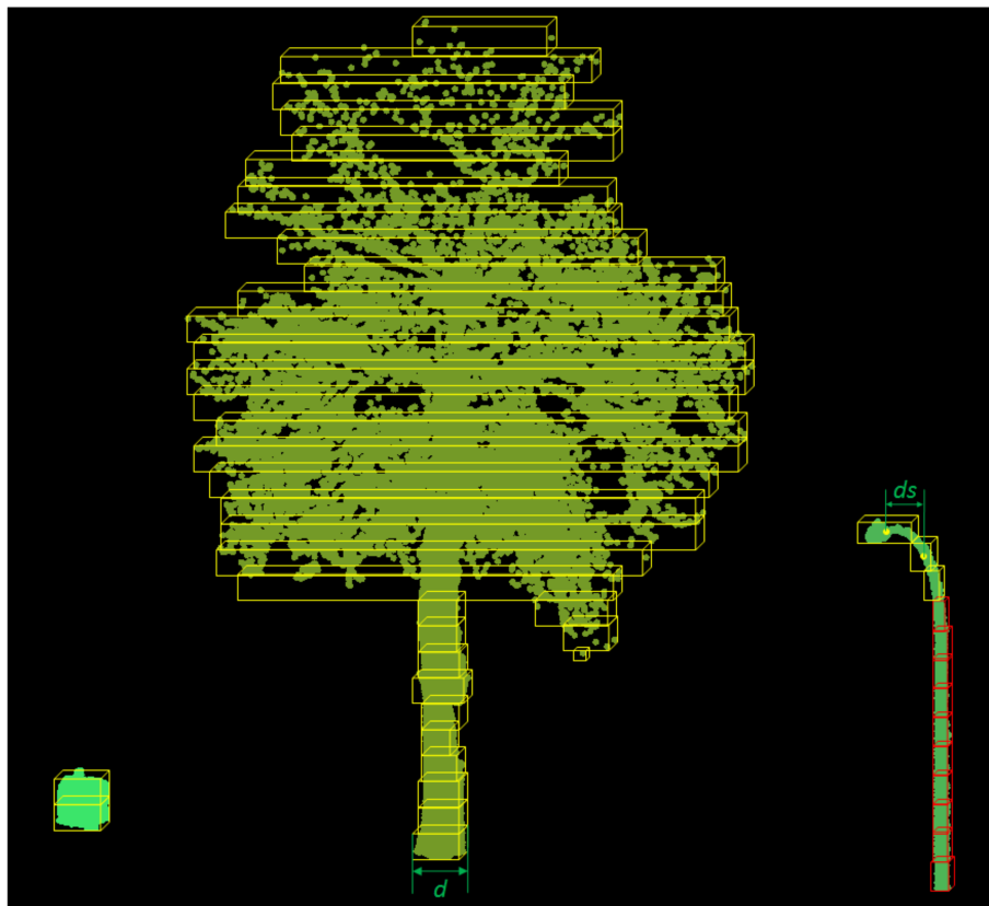
Figure 4. The slice-based detection of pole-like road furniture.
