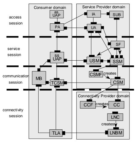
Figure 1: General MESH Release 2 architecture, showing software components, sessions and domains.
