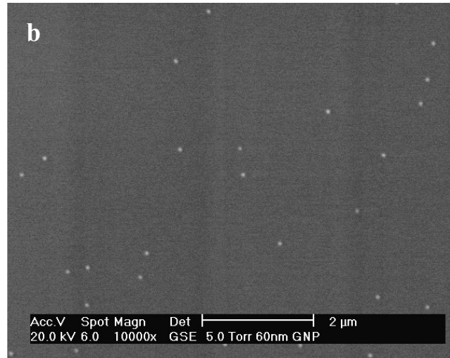
Fig. 6b. Typical ESEM image of BBI 60 nm GNPs immobilised on APTES coated glass slide
