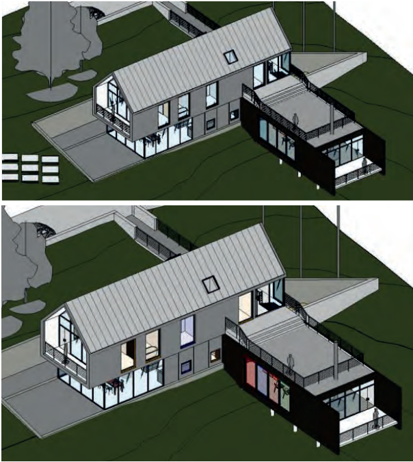
Figure 9 & 10: Colour feedback outputted by the host/hosted relation tool. By comparing the life span of walls and windows the tool can sort them into four different categories and change their displayed colours (b)
