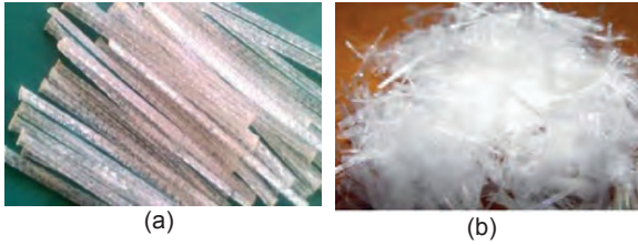
Figure 6: Forms of polypropylene fibers: a) twisted bundles, b) open continuous mesh.
