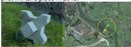
Figure 1 X-stream blocks and pilot location close to Kampen (Deltares 2017)
