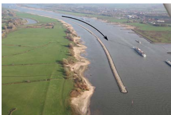
Figure 1: Aerial photograph of an LTD in the Dutch Waal River, which is used as prototype for the scale model. The arrow denotes the flow direction. (Courtesy: Rijkswaterstaat)
