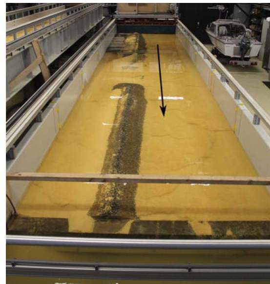
Figure 2: Scale model of the LTD with flowing water. The arrow denotes the flow direction in the main channel.
