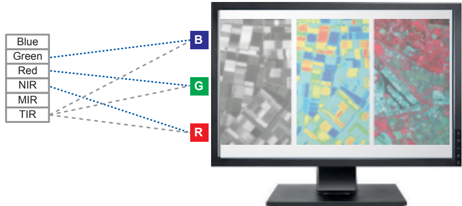
Figure 5.5 Single-band and three-band image display using the red, green and blue input channels of the monitor.
