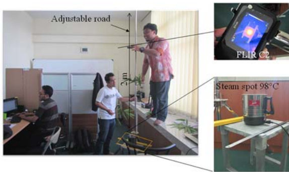
Figure 1. Experimental design using FLIR C2 at lab scale to measure a simulated steam spot using boiling water.
