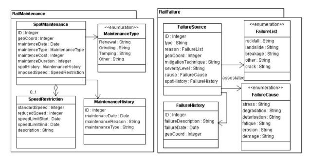
Figure 5: Information Model (Railway Maintenance) Figure 6: Information Model (Railway Failure)
