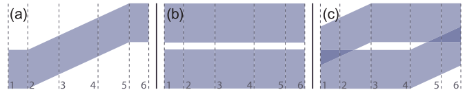
Fig. 3. Tape sections making up the geometry of the Roebel cable: (a) the cross-over bridge when located at the center of the unit cell, (b) the sloped tapes, and (c) the cross-over bridge at the edge of the unit cell.
