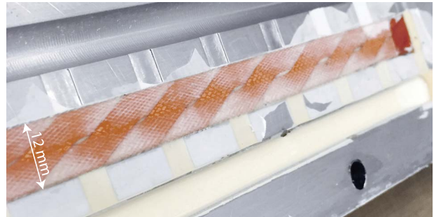
Fig. 7. One of the samples after impregnation with CTD 101G still inside its impregnation mold.
