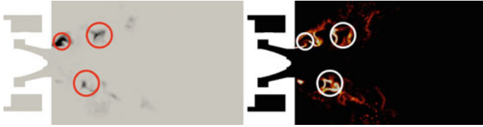
Fig. 2 Kerosene mass fraction ( left ) and heat release rate ( right ) and circles highlighting the influence of the PVC on the flame topology
