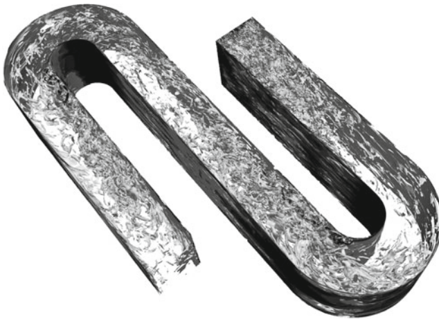
Fig. 4 DNS of serpentine flow using DGM and synthetic fluctuations. Vorticity iso-surfaces
