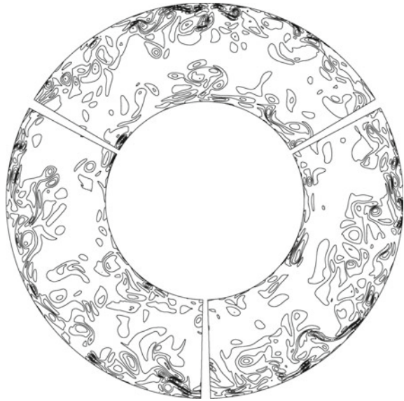
Fig. 6 Contour levels of streamwise vorticity in the reference case ( top part ), the forced convection case ( lower left part ) and the mixed convection case ( lower right part ). The contour levels are the same for all cases
