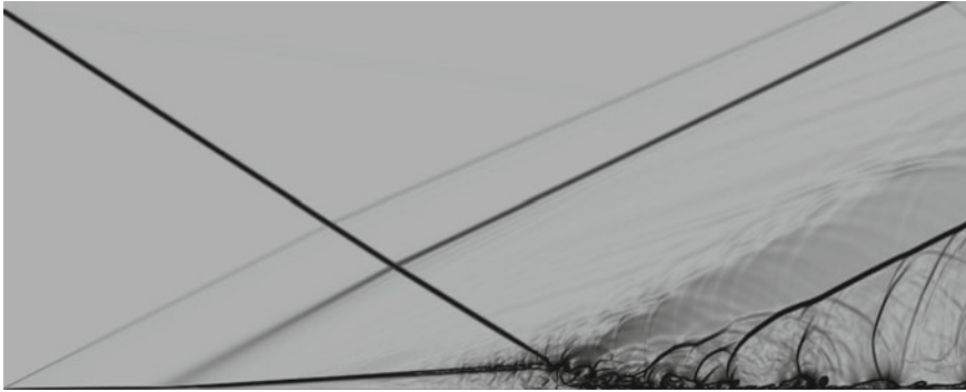
Fig. 1 Instantaneous contours of the numerical schlieren from a 2D simulations
