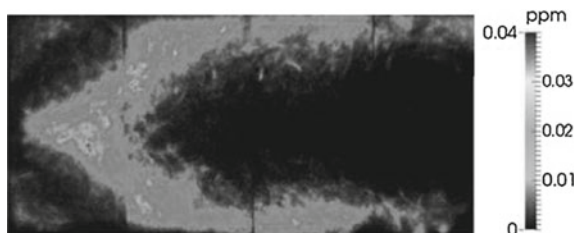
Fig. 7 Measured soot volume fraction
