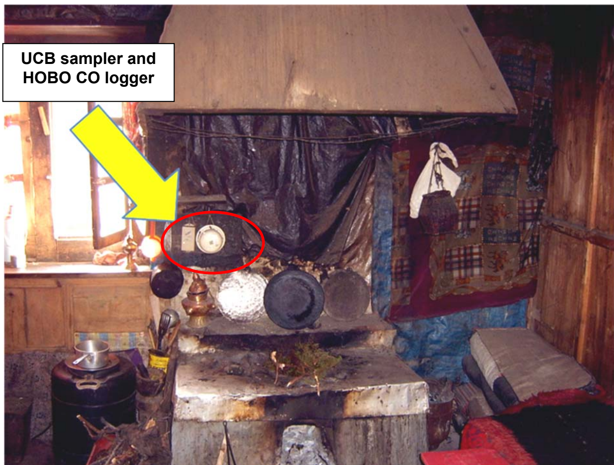
Figure 10: Measurement of CO and PM2.5 in tradition kitchen in Thame
