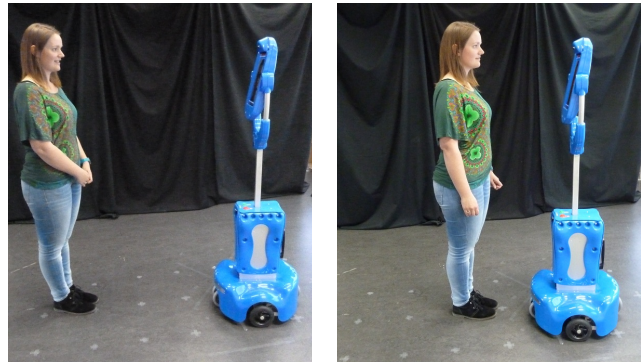
Fig. 1. The robot approaching the participant to a distance of 70-80cm (left) or trying to invade their personal space by using 30-40cm (right).
