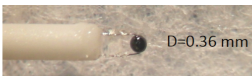
FIG. 3. Photograph of a type-111-104HAK-H01 (0.36-mm-diam) thermistor mounted through its 0.9-mm-diam ceramic rod. Adapted from Fig. 2 of Ref. [21].
