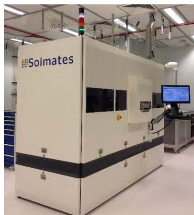
Figure 1. Solmates's Pulsed Laser thin-film Deposition (PLD) system in MESA+ NanoLab's cleanroom (University of Twente, The Netherlands).
