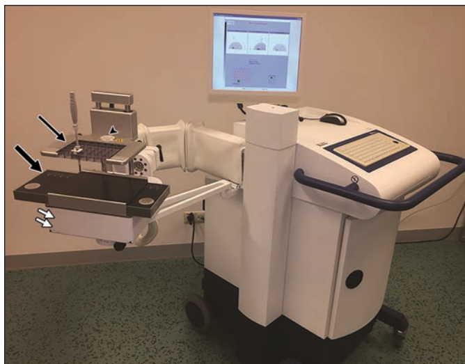
Fig. 1 —Molecular breast imaging–guided biopsy device equipped with compact stereotactic localization system containing fiducial source (arrowhead), grid paddle (thin black arrow), slant-hole collimators (thick black arrow), and detector (white arrows). Monitor displays breast images from two angles for calculation of x , y , and z coordinates of lesion and for determination of corresponding grid hole to insert needle.
