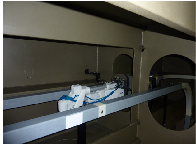
Fig. 12 Robot in experimental ballast water tank, with manipulator folded to a minimum volume
