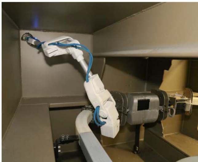
Fig. 11 Proof-of-principle manipulator, with covers, mounted on the robot, taking a measurement at one of the test locations
