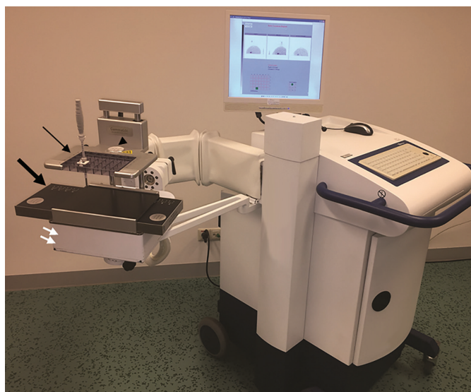
Figure 1. Molecular breast imaging-guided biopsy device equipped with compact stereotactic localisation system containing fiducial source (arrowhead), grid paddle (thin black arrow), slant-hole collimators (thick black arrow), and detector (white arrows). Monitor displays breast images from two angles for calculation of x, y, and z coordinates of lesion and for determination of corresponding grid hole to insert needle.
