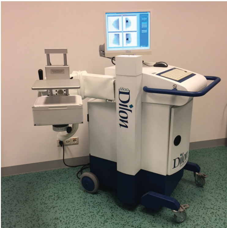
Figure 2. BSGI system is equipped with a single detector head and a compression paddle to immobilise the breast during image acquisition.
