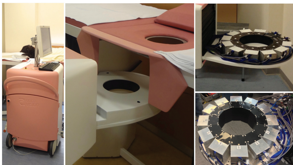
Figure 2. MAMMI-PET device for breast imaging with patient in prone position (on the left) with hanging breast configuration thanks to the special bed and ring camera (middle). On the right, internal view of the scanner showing a version with a single (top) and a double (bottom) full ring of detectors.
