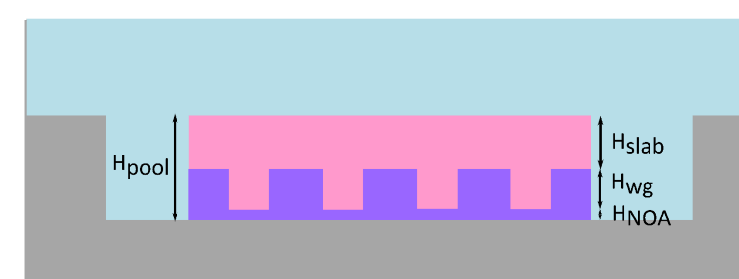
Schematic representation of the KYW substrate with waveguides after polishing.
