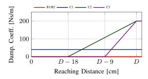
Fig. 2: Damping coefficients for each condition. Conditions B1 and B2 have zero damping coefficient. Condition C1 has a constant coefficient of 40 Ns/m. Conditions C2 and C3 increase linearly towards the target point from 0 Ns/m to 200 Ns/m.
