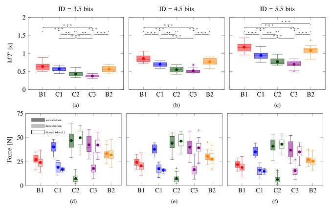
Fig. 6: Movement statistics. a–c) Movement Time MT. Statistical differences are only investigated between conditions and not between ID. Note that:  ${}^{(**)}p \leq 0.001$ ,  ${}^{(***)}p \leq 0.0005$ , and corrected significance threshold  $\alpha = 0.005$ . d–f) Modulus of mean acceleration force (left) and mean deceleration force (light colored, center) and mean device deceleration force (filled white, right) during a trial. For B1 and B2, there was no damper force from the device.
