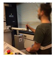
Fig. 3: A subject uses the Moog HapticMaster to move a cursor to a target shown on screen, while experiencing different kinds of damping forces.
