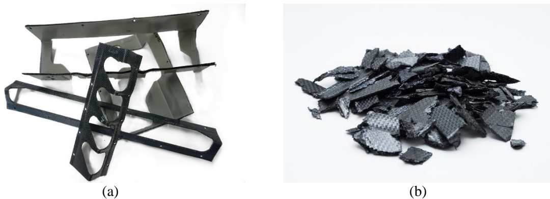
Figure 1: Pictures of C/PPS offcuts (a) and the outcome after shredding (b).
