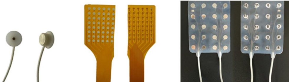
Figure 8.7 Various electrodes for sEMG measurements of the tongue. From left to right: micro electrodes (10 mm x 10 mm), high density grid (25 mm x 35 mm), ECoG grid (39 mm x 51 mm).
