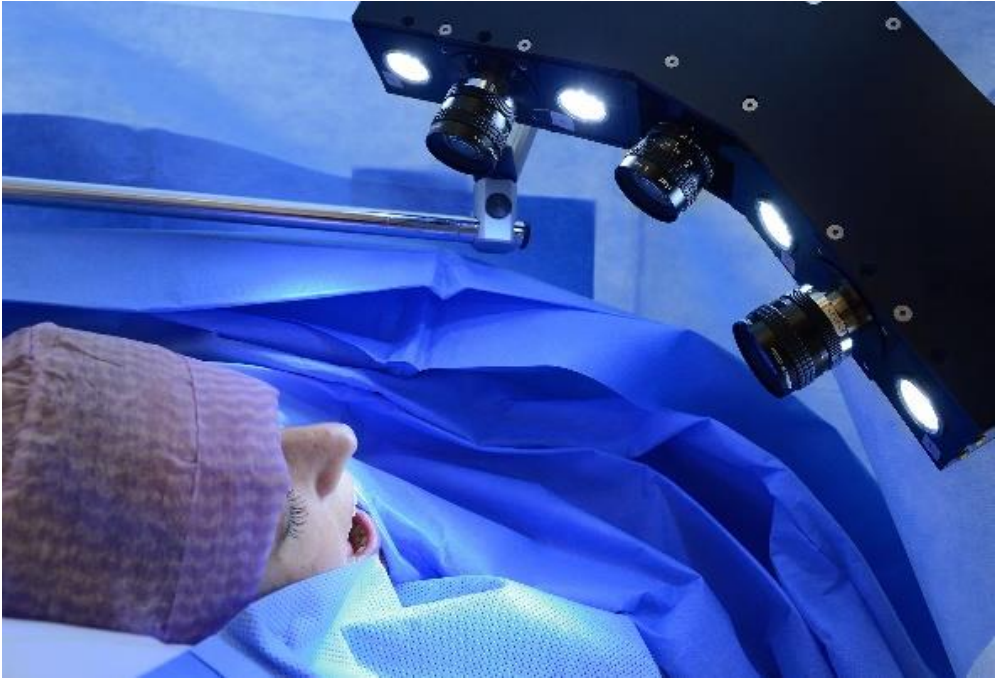
Figure 8.12 Triple-camera set-up able to acquire videos at 100 frames per second. Example perioperative image during in vivo nerve stimulation, simultaneously measuring artificially induced tongue movement, as was done in van Alphen et al. [8].
