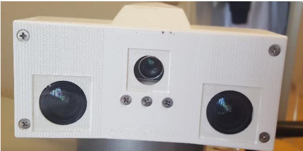
Figure 8.13 Stereo-camera set-up able to acquire videos at 50 frames per second and project images. Developed by Ferdinand van der Heijden and Kilian D.R. Kappert.
