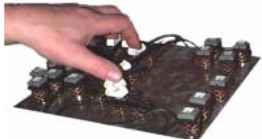
Figure 3. Flexipad with magnetic buttons and faders.
