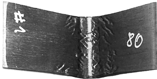
Figure 6.6 Ply wrinkling on the inner radius of a V-bend specimen (unidirectional carbon-PEKK). Reproduced from Sachs (2014) .
