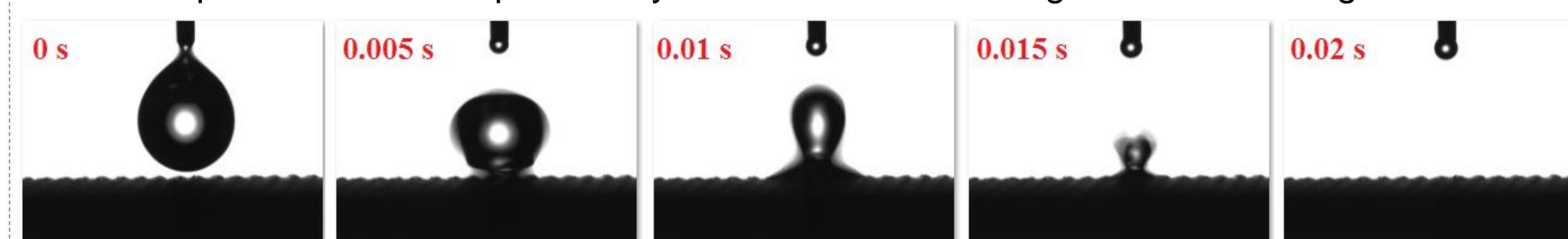
Instantaneous state photos of a deionized water droplet released onto the porous sample
