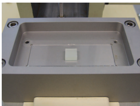
Fig. 2—Overview of the flat-on-flat contact between the silicone rubber test piece and the (coated) substrate.
