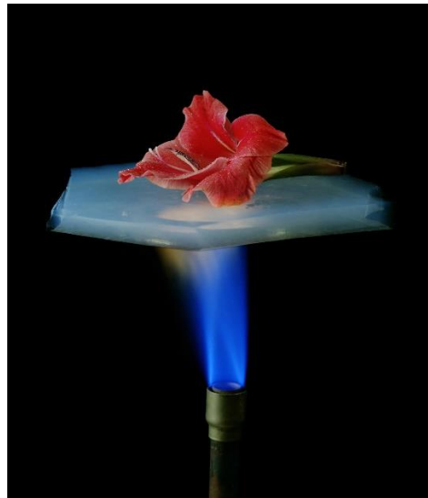
Figure 1.2 A photo showing the high thermal insulation performance of aerogel materials. The image was obtained from reference [19].
