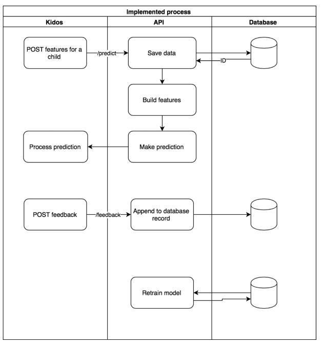
Fig. A7. Schematic view of the API implementation.
