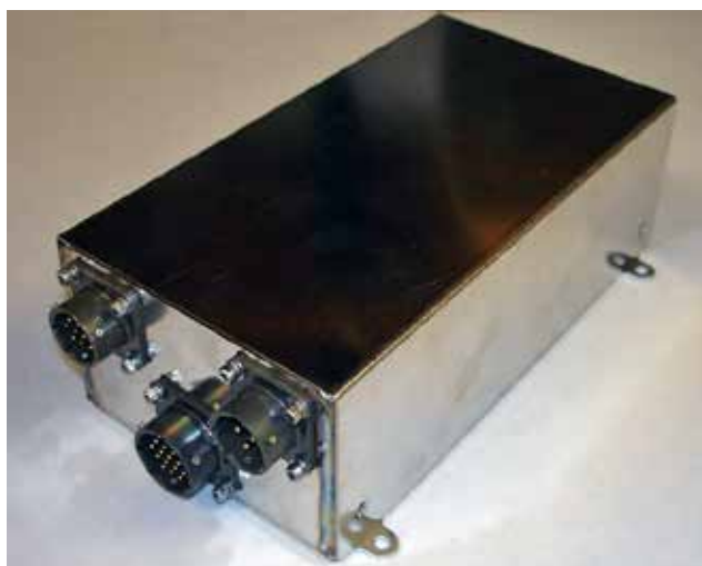
Figure 5: Shielded Enclosure (CB type III) with Connector Plate (CB type I)
