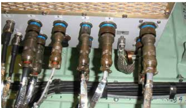
Figure 3: Connector Plate (or CB type I) as part of a Shielding Cabinet
