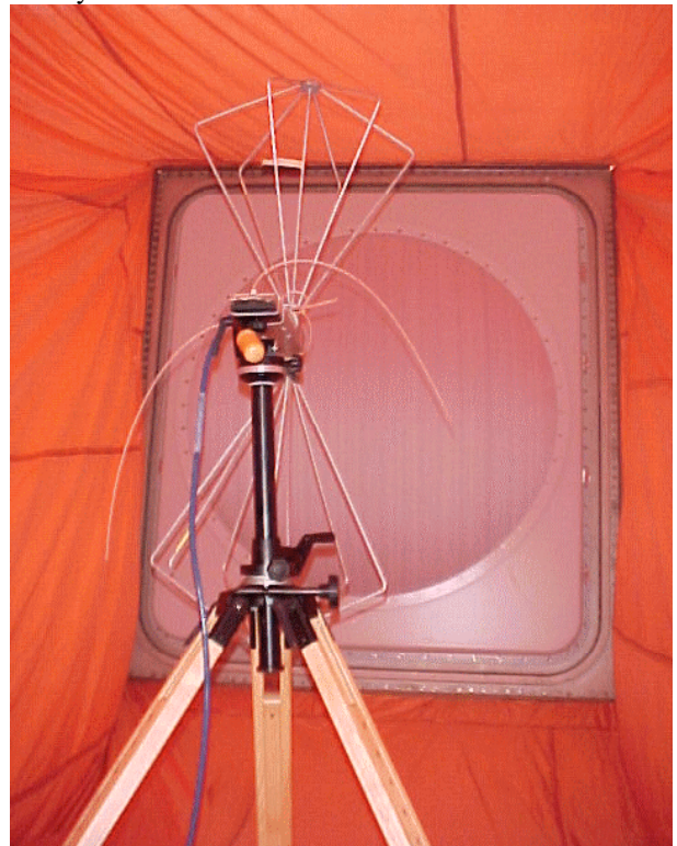
Figure 18: Test set-up: EUT in the VIRC, with an antenna placed in foreground
