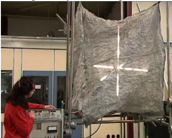
Figure 3: Three fluorescent tube lights in the VIRC, at 3 GHz and 50 W injected power.
