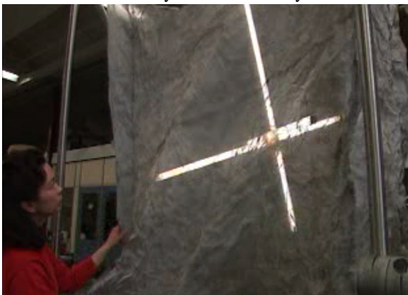
Figure 5: Due to the vibration of the walls the light intensity is constant over the volume of the VIRC.
