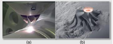
Figure 1: Directed energy deposition [1] (a), Powder bed fusion [2] (b)
