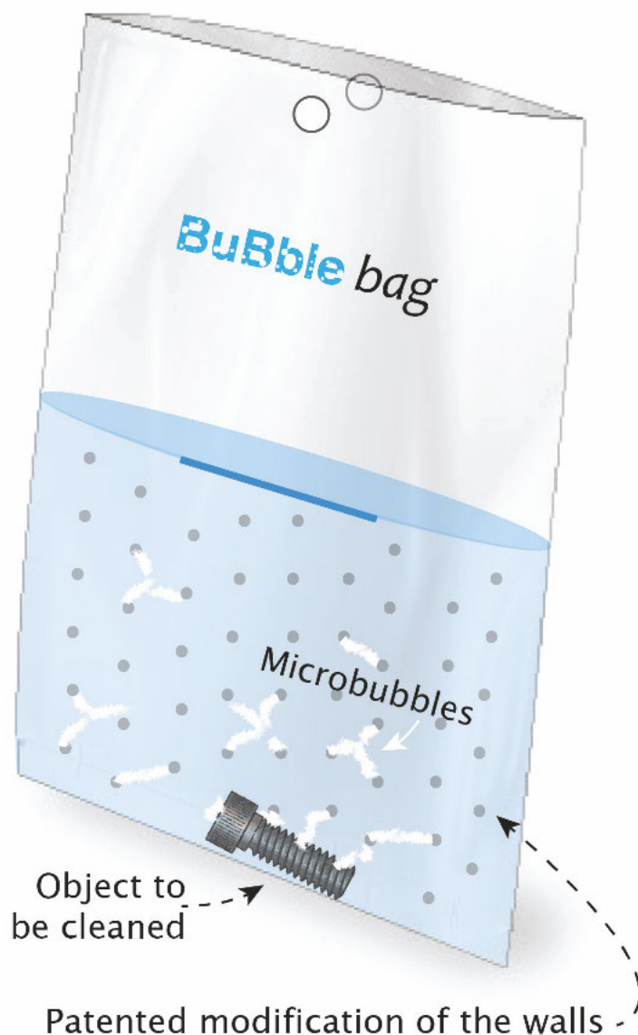
<< Figure 1: Picture of the BuBble bags in which modification of the internal walls leads to improved bubble formation for cleaning. >>
