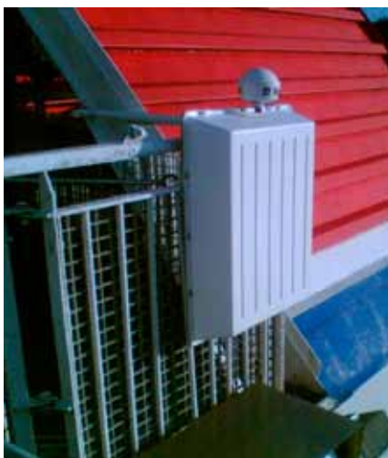
Figure 2-14: Antenna in radome and DGPS
