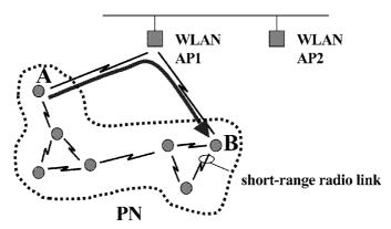
Figure 4. Infrastructure-oriented routing.
