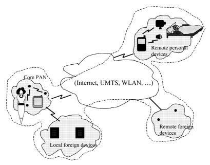
Figure 2. Components of a Personal Network.
